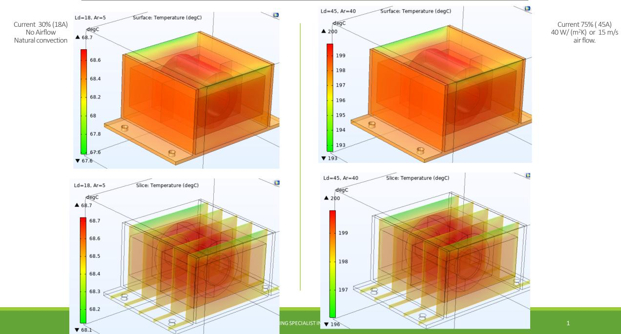
Thermal and Electromagnetics simulation – Part # EEK55246-171M-60A – Current rated 60A @ 10kHz
