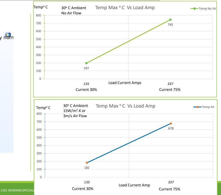
Thermal and Electromagnetics simulation – Part # HCS-631M-450A – Current rated 450A @ 10kHz
