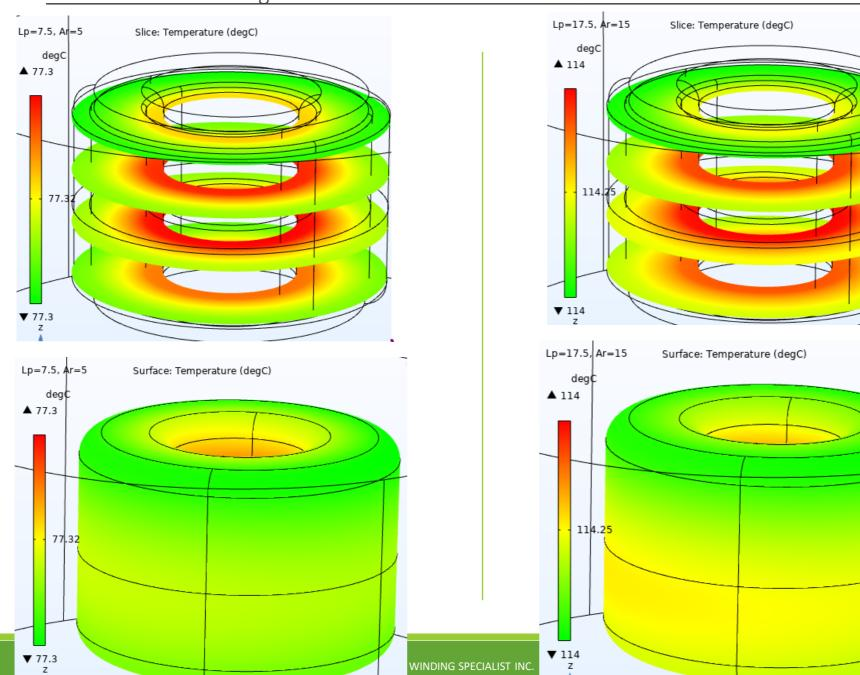
Current 30% (7.5A) No Airflow Natural convection Current 70% (17.5A)  $15 \text{ W/ (m}^2\text{K) or } 3 \text{ m/s}$  air flow.
