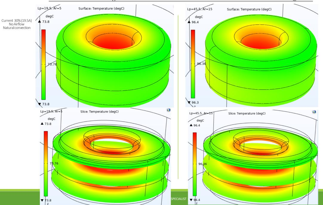
Current 70% (45.5A)  $15 \text{ W/ (m}^2\text{K) or } 3 \text{ m/s}$  air flow.
