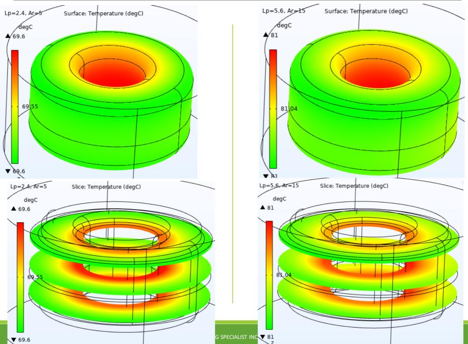
Current 70% (5.6A)  $15 \text{ W/ (m}^2\text{K) or } 3 \text{ m/s}$  air flow.
