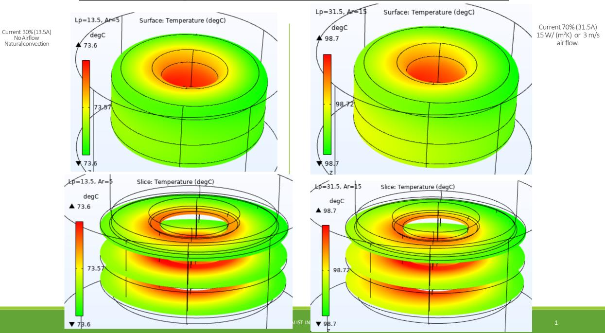
Thermal and Electromagnetics simulation – Part # HF467-260M-45AV – Current rated 45A @ 1kHz
